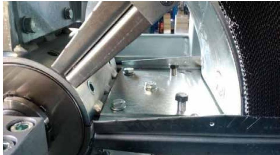
Insert the four M6x16 bolts into the openings in the sheet at the periphery of the rotor and tighten them.
