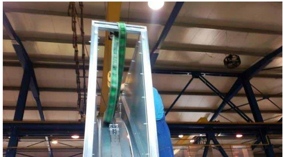
Using a crane, place the upper half of the casing onto the lower half.
