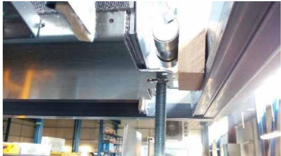
The sheet steel from the casing of the lower half of the rotor must be pushed between the storage mass and the casing of the upper half of the rotor.
